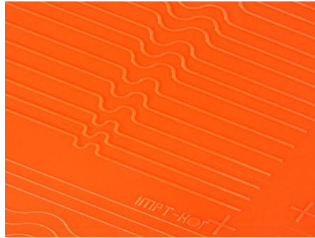
Figure 5.26: Microscope image of a PDMS soft stamp for waveguide fabrication.
