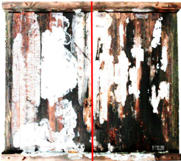
Figure 3. Scots pine sapwood (left) and Douglas fir heartwood (right) exposed in a Double layer test for 7 years.
