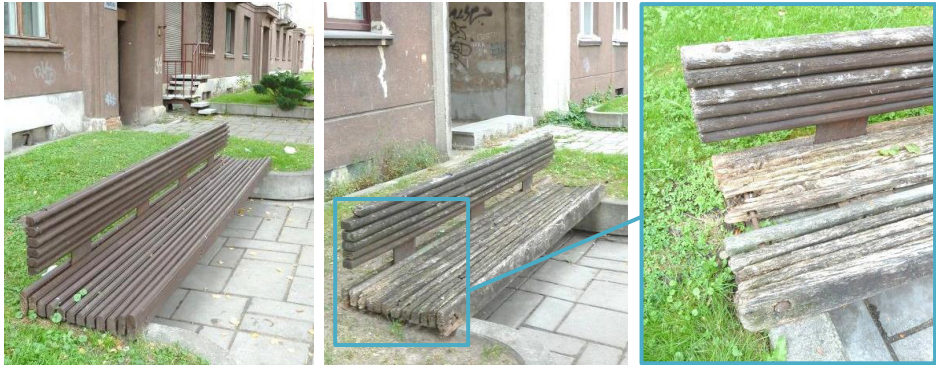
Figure 4: Bench in the city of Kaunas, Lithuania. Exposure in UC 3.2, close to the ground. Left: Newly installed bench. Middle: Bench after exposure. Right: Detail of bench severely decayed after exposure for several years.
