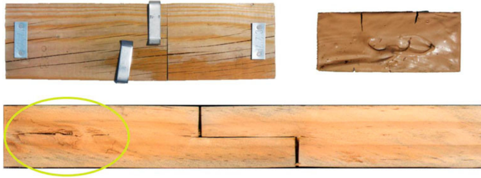
Figure 6. Top left: Lap-joint specimen after 3 months of exposure; top right: cracks have already led to damages in the end-grain sealing. Bottom: slide cut from Lap-joint specimen exposed for 3 years, showing heavy decay inside the specimen close to the end grain.
