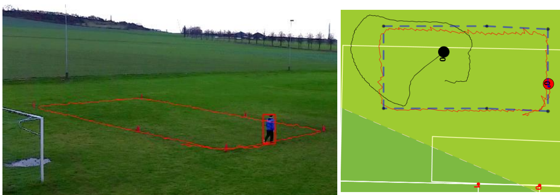
Figure 8. The resulting trajectories of the accuracy experiment: GPS (black) and result of our approach (red). The dots are the object current position determined by GPS (black) and our approach (red). The ground truth polygon is marked by a dashed blue line.
