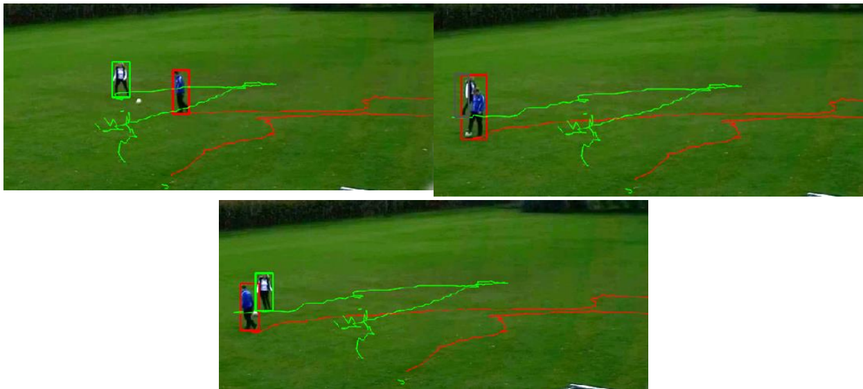
Figure 11. Another situation where the person marked green is occluded for about 1.5 s (8 frames). The assignment is continued correctly after the situation has cleared up.
