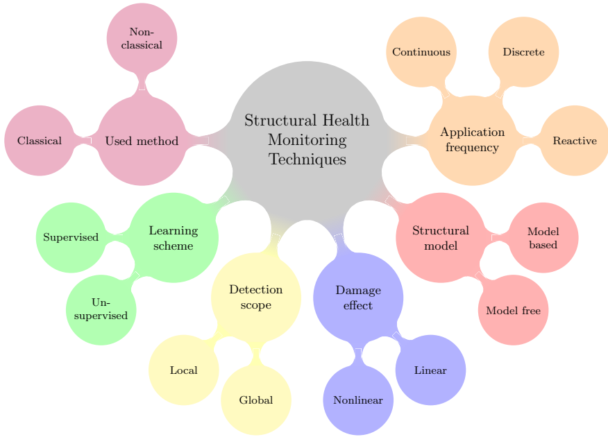
Figure 1.3: Classification of structural health monitoring problems.
