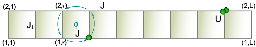
Fig. 6.4: Bosons on a two-leg ladder in the presence on a homogeneous flux \phi per unit cell with a rung-hopping J_{\perp} and the leg-hopping J (6.14).
