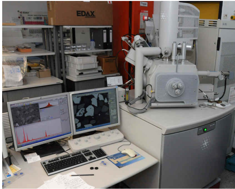
Figure 7.2: The FEI Quanta 600 FEG environmental scanning electron microscope with Mineral Liberation Analysis software in operation at BGR, Hannover. The left screen is showing an EDX-spectrum of an analysed mineral grain and the right screen displays the BSE image of the scanned sample surface.
