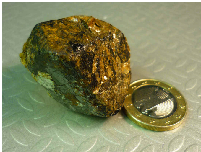
Figure 3.2: Euhedral cassiterite crystal from the El Karit hydrothermal vein deposit, Morocco with coin (1 €) for scale. Specimen is taken from the BGR mineral collection.
