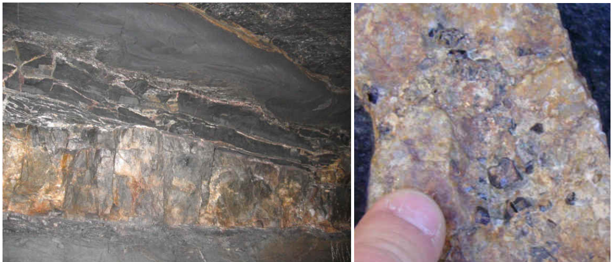
Figure 6.13: Sn-W mineralised vein deposits. Left picture: Reinite-bearing quartz vein crosscutting graphitic phyllites from the Nyakabingo mine, Rwanda. Right picture: Large cassiterite crystals in quartz vein from Krupka, Czech Republic.
