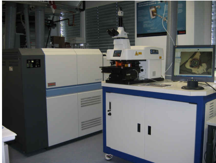
Figure 7.4: The LA-ICP-MS system in operation at BGR, Hannover. The New Wave UP193-FX laser ablation unit is shown on the right hand side with the ATLEX-300-SI excimer laser stored in the cabinet below. The screen displays the ablation pit of the laser on a columbite-tantalite grain. The Thermo Scientific ELEMENT-XR mass spectrometer is shown on the left hand side.
