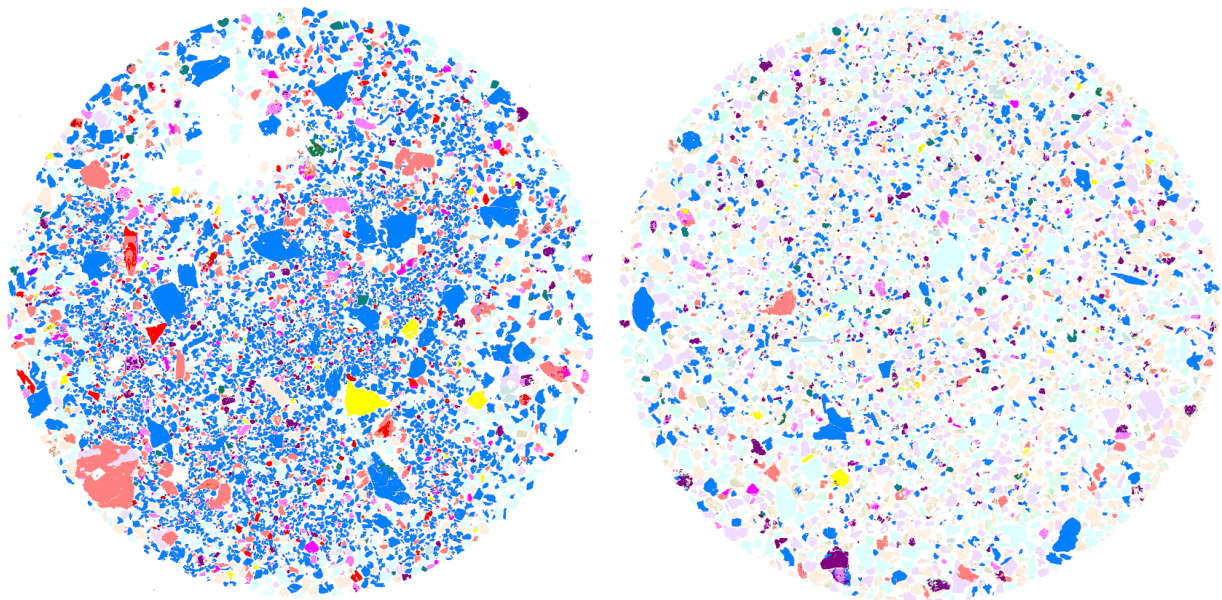
Figure 11.1: MLA images of two heavy mineral concentrates from Simba, Rwanda. Different colours represent different mineral phases: e.g., cassiterite (blue), columbite-tantalite (pinkish and red), rutile (yellow), topaz (pale blue), muscovite (pale green), quartz (pale violet) and Fe oxides (apricot). Comparison of these two MLA images reveals the different ore grade of the two concentrates although they originate from the same deposit: 46.7 area% cassiterite (left) versus 12.7 area% cassiterite (right).
