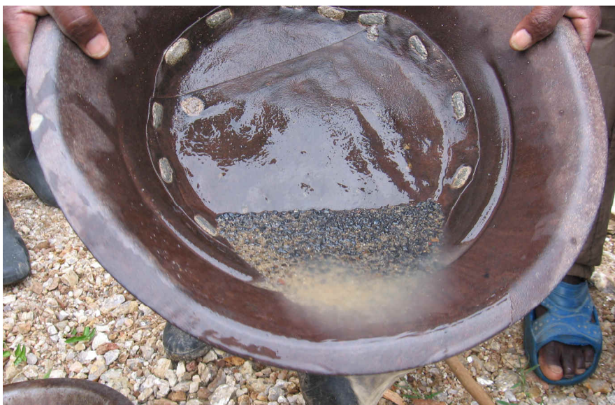
Figure 7.1: Heavy mineral pre-concentrate from Rukaragata pegmatite in Rwanda. This pre-concentrate is essentially composed of cassiterite and columbite-tantalite (black grains).
