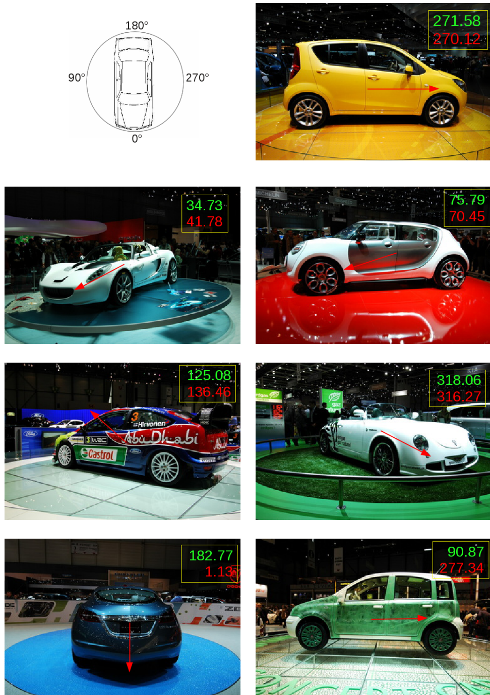
Figure 4.11: Results of our method on the EPFL car dataset. In the top left corner, a diagram representing the car orientation, where the car front is labeled by 0^\circ . For each picture, the ground truth value (green) and the estimated one (red) are given in a box and a red arrow is overlaid on the car. In the last row, two examples of flipped estimation are provided. The pose of the car in the bottom left corner is hard to guess also for a human being.
