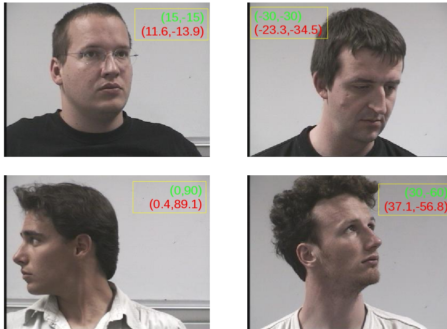
Figure 4.12: Results of our method on the Pointing'04 face dataset. In this case, the returned pose value is two-dimensional, as it is given in terms of pitch and yaw. The ground truth pose (green) and the estimated one (red) are given in a box.
