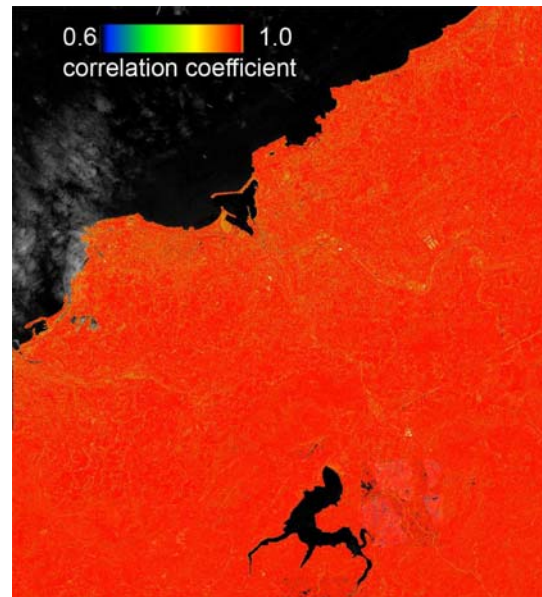
Figure 7. Distribution of correlation coefficients in scene combination centre and last image laid over Pleiades image
