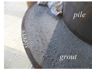
Before testing: No visible cracks, conspicuous air bubbles arised during hardening process
