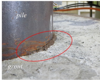
LS03: Powdery rust-coloured cementitious material
