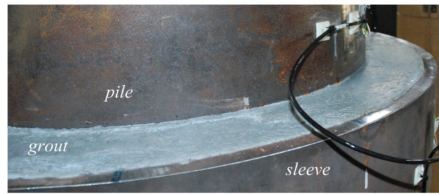
Before testing: No visible cracks
