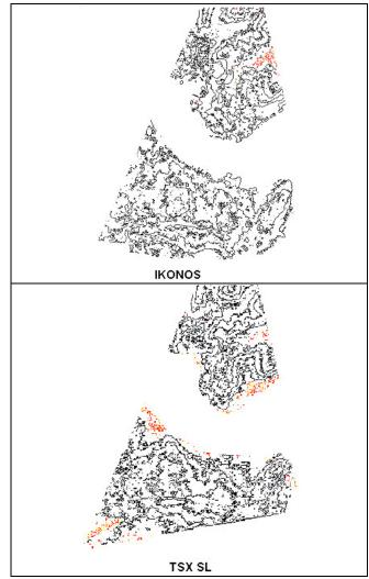
Fig. 13: Contour lines of IKONOS and TSX SL DSMs with 20m contour interval
