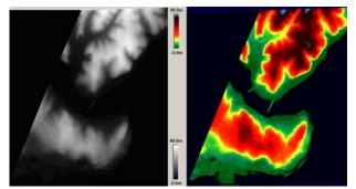
Figure 8. Grey value and color coded reference DEM
