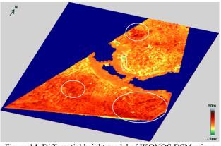
Figure 14. Differential height model of IKONOS DSM minus TSX SL DSM
