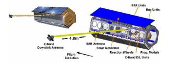
Figure 2. System components of TSX
