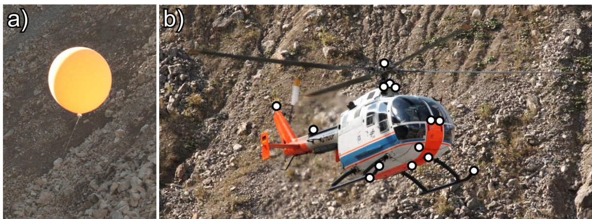
Figure 5.17: Photographs of a) a large helium balloon, and b) the BO 105 with selected marker positions for the camera calibration
