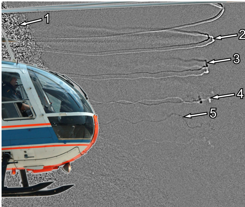
Figure 5.7: Photograph of the BO 105 in hover with overlaid BOS result depicting vortices up to \psi_v = 450^\circ and vortex instability effects, after Bauknecht et al. (2014a).
