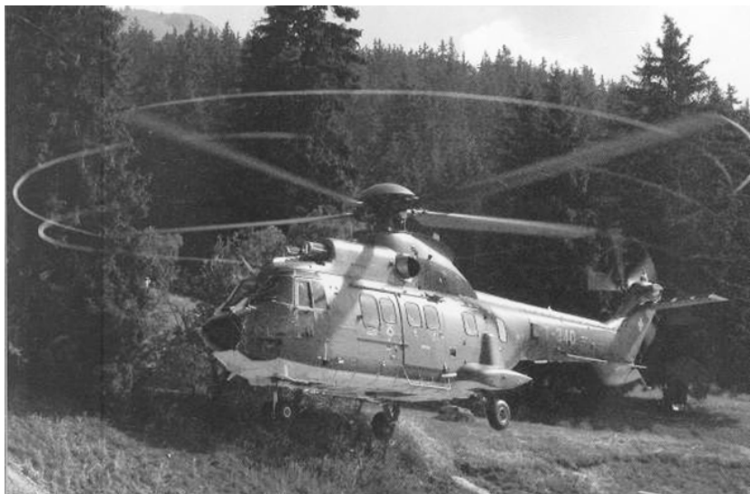
Figure 5.1: Natural condensation on a Cougar helicopter, after Leishman (2006)
