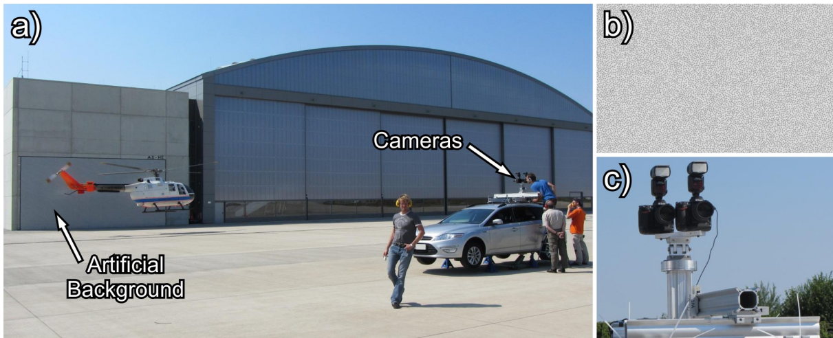
Figure 5.6: Photographs of the reference-free BOS hover test with a) test overview, b) artificial background pattern, and c) dual-camera setup, after Bauknecht et al. (2014a)
