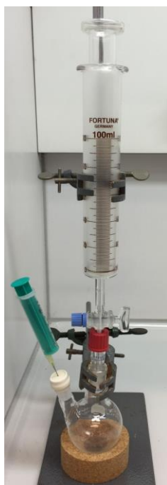
Figure 2.7: The glass apparatus used for ACHR experiments
