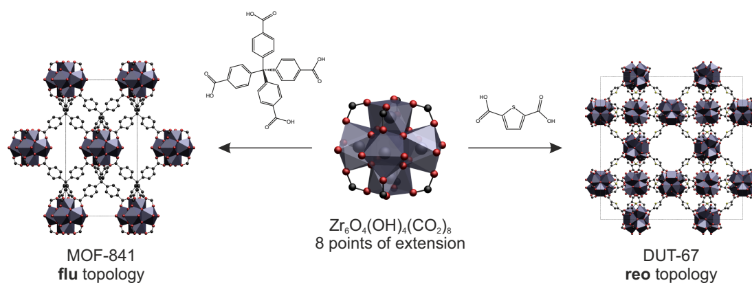
Figure 4. Reaction of a metal cluster/Zr-IBU with different multitopic ligands results in different network topologies. Crystal structures depicted are from references 32, 33.
