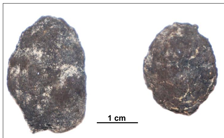
FIGURE 4.1 Typical small nodules which were taken for high resolution computer tomography analysis. These nodules show slightly botryoidal rough growth structure on every side.
