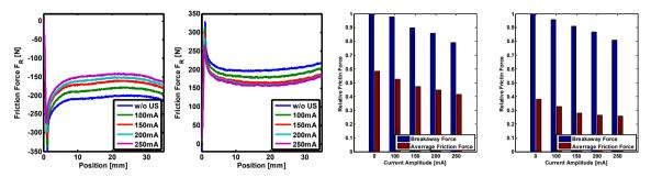
Fig. 4. (left ) Force-Position diagram for contracting actuator. (middle left) Force-Position diagram for expanding actuator. (middle right) Relative Friction force for expanding actuator. (right) Relative Friction force for contracting actuator.
