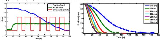
Fig. 3. (left) Transient behavior of novel ultrasonic pneumatic actuator. 0.75 bar air pressure. (right) Variation of current amplitude.
