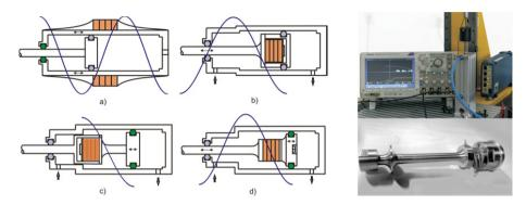
Fig. 2. (left) Concepts for integration of ultrasonic transducer in pneumatic actuators. (right bottom) Ultrasonic Piston. (right top) Universal Linear Force-Displacement Test Bench for Characterization.
