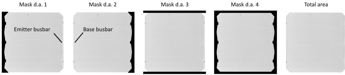
Figure 6.8: Sketch of the masks used for determination of the effect of busbar and edge regions on the cell performance. The cells are measured in the I - V with the shadow masks on their front side. Here, the rear side of a BJBC solar cell is shown to illustrate the location of the mask with respect to the doping geometry, which coincides to the metallization geometry for this cells.
