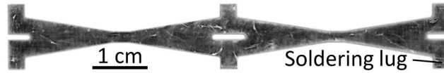
Figure 6.23: Interconnect as used for laser soldering of 125 \times 125 \text{ mm}^2 BJBC solar cells.
