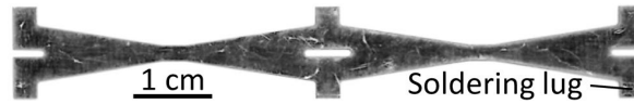
Figure A.1: Interconnect as used for laser soldering of 125 \times 125 \text{ mm}^2 BJBC solar cells.
