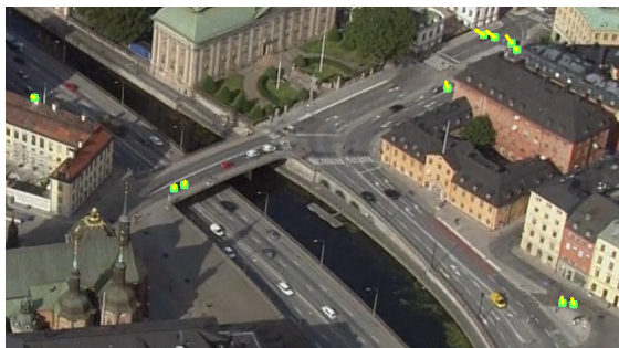
(a) Stockholm, cluster filter. Sometimes mis-detection of slowly moving vehicles (green dots).
