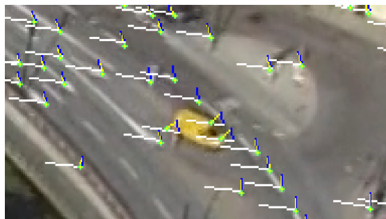
(b) Stockholm, motion parallax predictor classifier. Slow vehicles are not detected if they move along the predicted epipolar line segment (green cross close to the white line at the yellow van).
