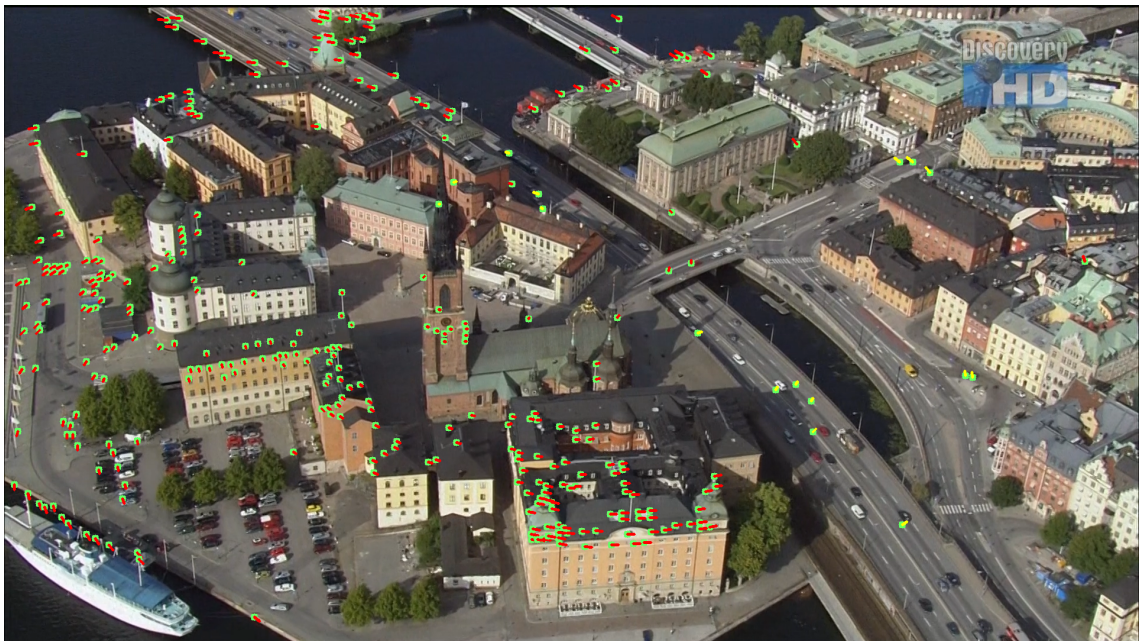
(b) Stockholm, fundamental matrix classifier. Unreliable determination of the F-matrix results in large areas of false classifications (false positives as well as false negatives).
