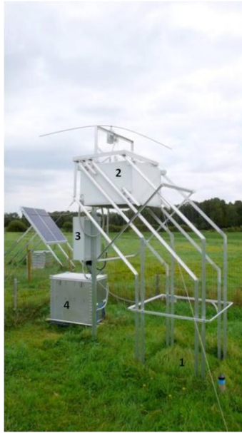
Fig. 2 - 1: Photograph of the automatic chamber system (chamber in standby position). Numbers indicate the most important components: soil frame (1), measurement chamber (2), box with control unit, data logger and CO 2 analyzer (3), box with vial sampling system (4).
