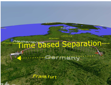
Figure 3.3 – Time-based Separation between 4D-Trajectories
