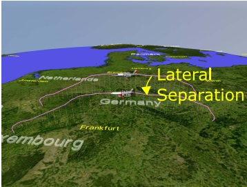
Figure 3.1 – Lateral Separation between 4D-Trajectories
