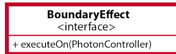
Figure 4.21.: A plugin which should act as boundary effect has to provide the BoundaryEffect service connector.
