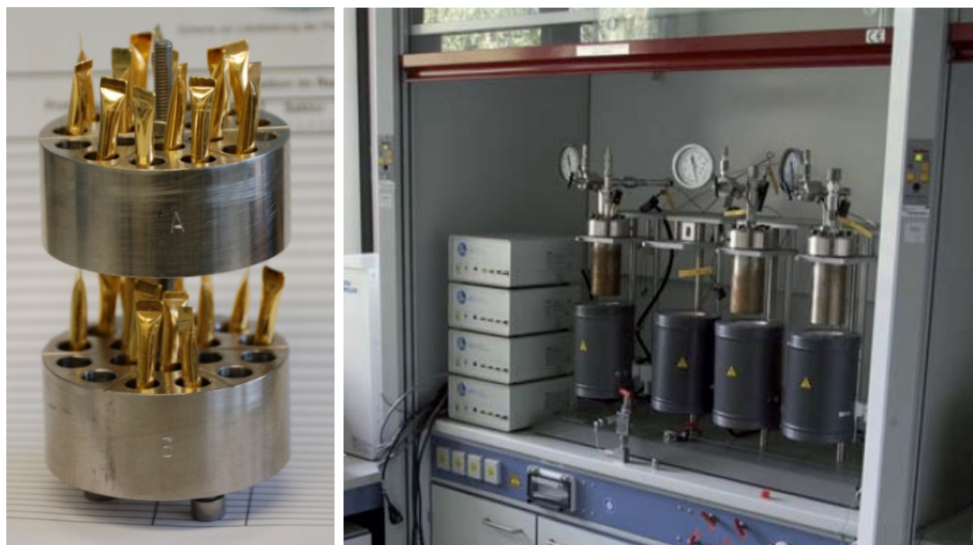
Fig. 14: Samples in the sample holder (left), which can be loaded into the Parr hydrothermal reactor (right). In the right picture all reactors are not running. This is represented by the ovens that are not covering the reactors. (photographs taken by Christian Ostertag-Henning)
