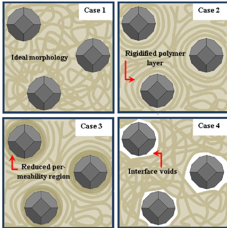
Fig. 6: The schematic diagram of various morphology of the mixed matrix structure.[22] Case 1 is the ideal case without morphology changes; case 2 shows a rigidified polymer due to the incorporation of filler particles; case 3 shows a reduced permeability region on the surface of the porous filler particles and case 4 illustrates the void-forming between the polymer matrix and the filler particles.
