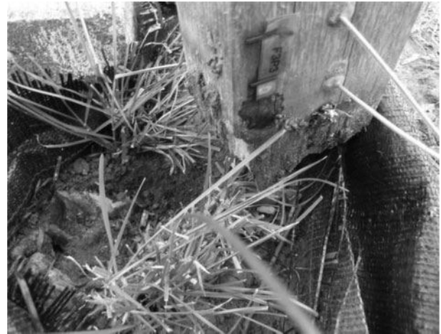
Figure 9. Failure of a fence post on the ground area made from Norway spruce after 4 years exposed at the test field of the IBW in Hannover, Germany.
