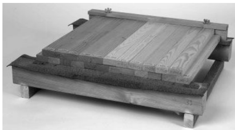
1 Double layer test rig with upper specimen layer shifted by 25 mm horizontally to lower layer: specimens are separated with bitumen foil from chromium-copper-boron (CCB) impregnated support beams
