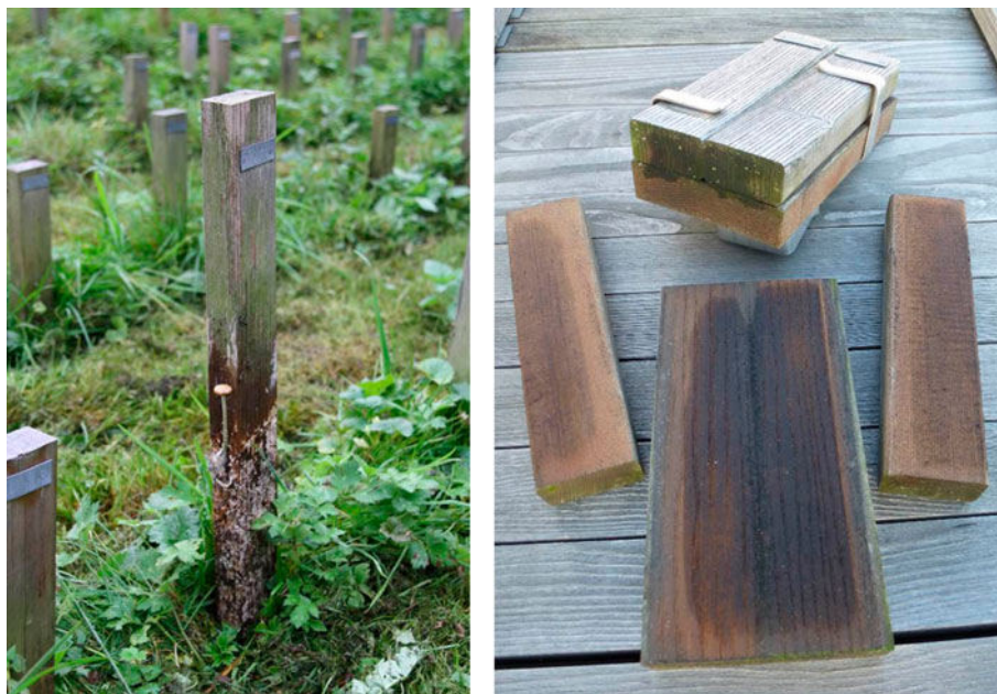
Figure 2. Testing thermally modified ash ( Fraxinus excelsior L.) in the field under differently severe exposure conditions in Hannover, Germany. Left: severe white rot decay after 2.5 years exposure in ground according to EN 252 (CEN 1989). Right: sandwich specimen after 2.5 years above ground exposure without signs of decay (Photos: L. Meyer & Ch. Brischke)
