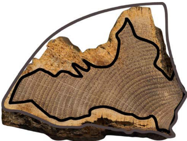
Fig. 2 Determination of remaining cross section. Grey line : Reconstructed original heartwood cross section. Black line : Remaining undecayed heartwood cross section
