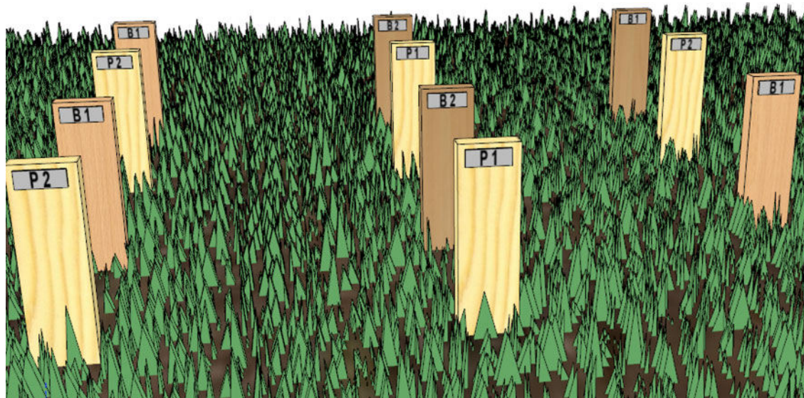
3 Position of specimens: P1, Scots pine sapwood exposed in the first year; P2, Scots pine sapwood exposed in the second year; B1, beech exposed in the first year; B2, Beech exposed in the second year
