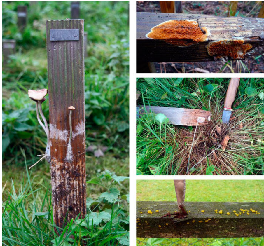
Figure 3. Examples of rot causing fungi not represented as obligatory test fungus in recent European standards, but frequently found on field test samples and timber structures. Left: white rot by Hypholoma sp. on Douglas fir heartwood ( Pseudotsuga menziesii Franco.) exposed in ground in Hannover, Germany (Photo: L. Meyer). Right top: brown rot by Serpula himantoides on buried test stake at Oléron test site, Southern France (Photo: R. Gründlinger). Right centre: brown rot decay by Leucogyrophana pinastri on Scots pine heartwood ( Pinus sylvestris L.) exposed in ground in Hannover, Germany (Photo: L. Meyer). Right bottom: brown rot on above-ground exposed thermally treated beech ( Fagus sylvatica L.) after eight years exposure caused by Dacrymyces sp. (Photo: Ch. Brischke)
