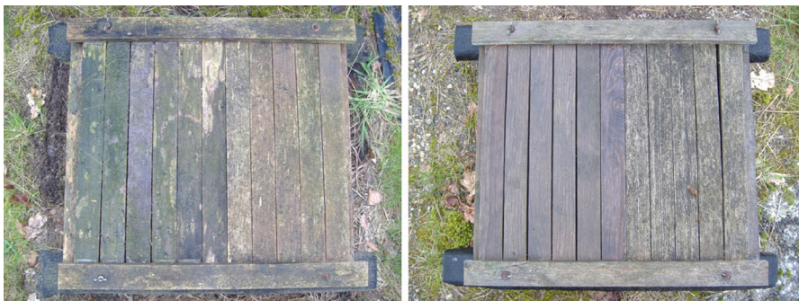
Fig. 6 Double layer test set ups after 6 years exposure in Hamburg, Germany, in artificial shade (left) and exposed to the sun (right). Algae are growing on the upper surface of the shaded Douglas fir heartwood and Scots pine sapwood specimens
