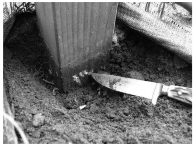
Figure 10. Decay on a fence post on the ground surface area made from Douglas fir after 3 years exposed at the test field of the IBW in Hannover, Germany.
