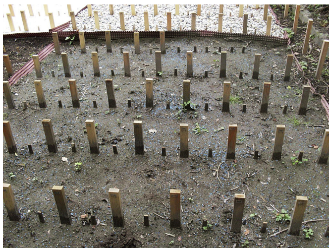
Fig. 2. Alternating order of mini stake and standard specimens according to EN 252 (1989).
