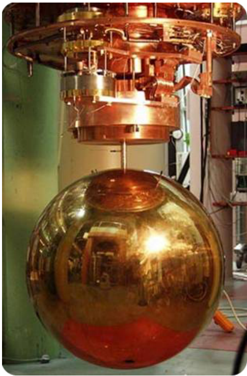
Figure 1.3: MiniGrail, the first spherical GW detector, is operating in 2 – 4 kHz high frequency range at Leiden University in the Netherlands.
