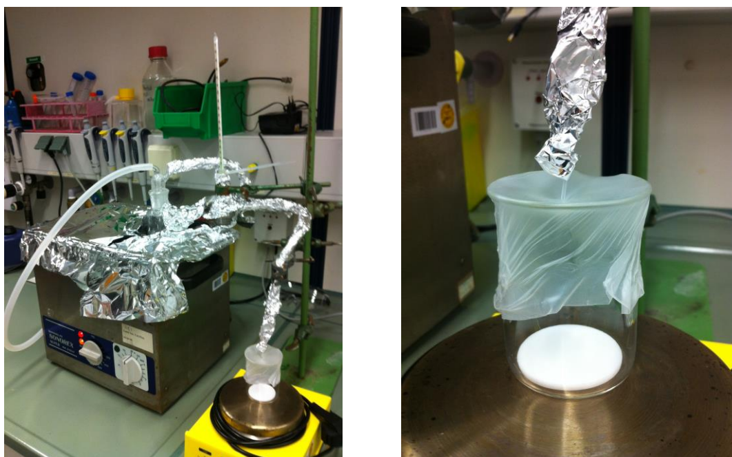
Figure 80: A glass flask and a water bath were used to heat up nitrogen and enrich it with water. The jet was then directed to the beaker with the Teflon disk to prehydrate the lipids.
