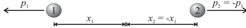
Figure 2.1.: Correlated particles. In their famous thought experiment, Einstein, Podolsky and Rosen considered two particles from a common source with opposite position and momentum.
