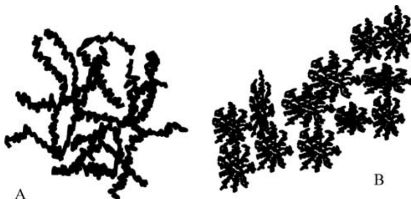
Figure 1.13: A cartoon showing linear weakly cross-linked and highly branched clusters, A: acid catalyzed B: base catalyzed hydrolysis.
