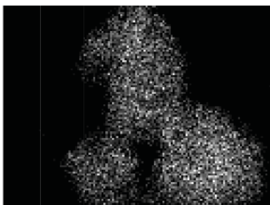
Figure 7: TEM micrograph of an agglomerate of crystallites of \text{Ba}_{0.60}\text{Ca}_{0.40}\text{F}_2 (a) and the spatial distribution of fluorine (b), Ca (c) and Ba (d) in it.
