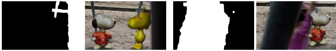
(a) Color similarity of foreground and background (b) Smeared object boundaries due to motion blur
