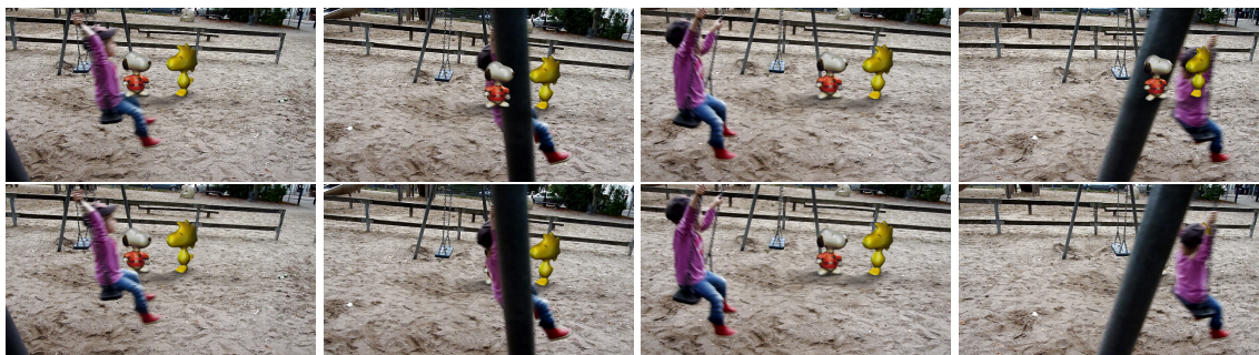
Figure 5.7: Playground sequence from Figure 5.1, As shown in the top row, for integrating virtual objects, it is essential to handle foreground occlusions in the composition of virtual and real scenes. The desired result should look like in the bottom row: the integrated virtual objects are occluded accurately and reliably [25].
