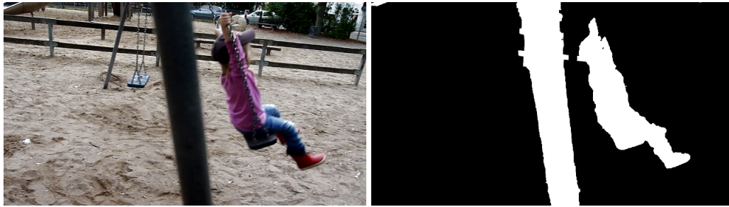
Figure 5.8: Binary segmentation of the input image (left) into two classes: Foreground and background, illustrated with the colors white and black, respectively.
