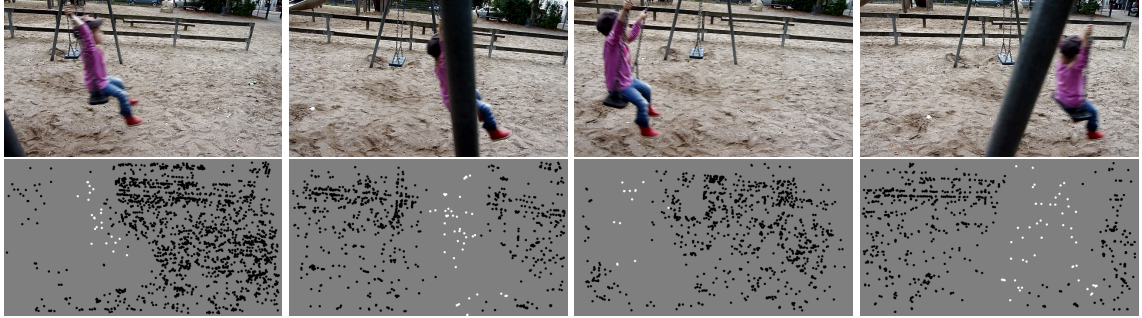
Figure 5.6: Visualization of the occlusion information of the Playground sequence (images k = 12, 34, 45, 77 ) from Figure 5.1: occluded (white) and not occluded (black) object points interpreted as foreground and background regions [25]
