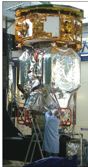
Figure 1.24: A photograph of the satellite and propulsion module. Photo courtesy of ASD.
