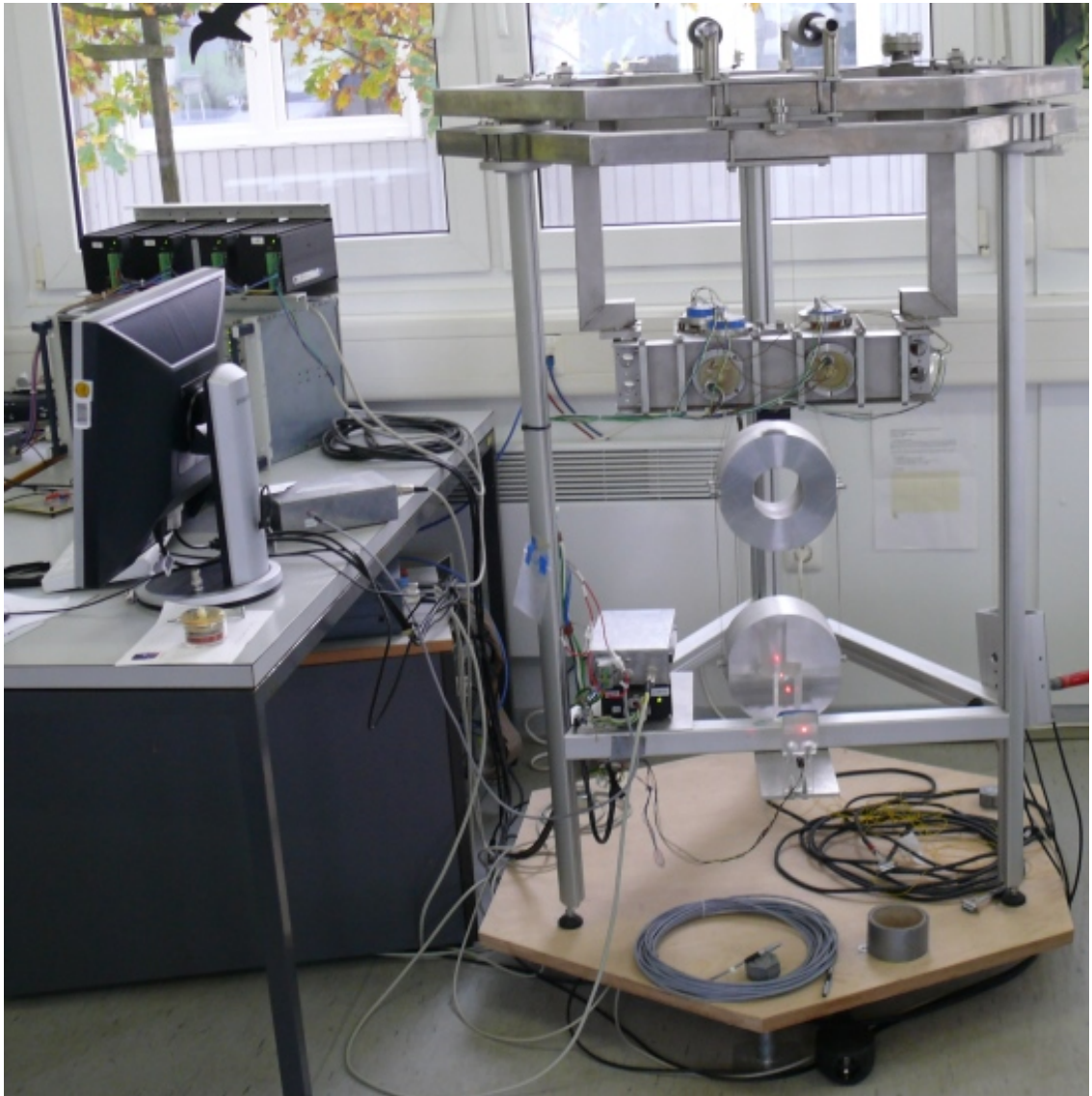
Figure 3.11: The GEO 600 test suspension. This is a duplicate of a GEO-like triple suspension including a six channel local control system. Initial experiments with the MD were performed at this test setup.
