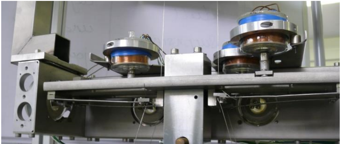
Figure 3.3: A photograph of the flag assembly at a GEO like suspension model. Metal flags attached to the upper mass stick into the glass housing of the coils. There is sufficient space between a flags and the corresponding glass housing for scattered light to enter.. Because the shadow sensors are encapsulated inside the glass, the scattered light can eventually reach them.
