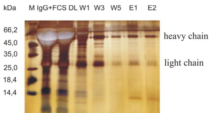
Figure 3.2.6 3: SDS PAGE analysis of the purification of IgG from 10% FCS utilizing aptamer 264 with integrated spacer and NHS-activated sepharose. Following samples were applied: (M) molecular weight marker, (IgG + FCS) IgG (from 10% FCS) sample applied to aptamer-modified sepharose, (DL) supernatant of IgG (from 10% FCS) after incubation with aptamer-modified sepharose, (W1-W5) washing fractions, and (E1-E2) eluates.
