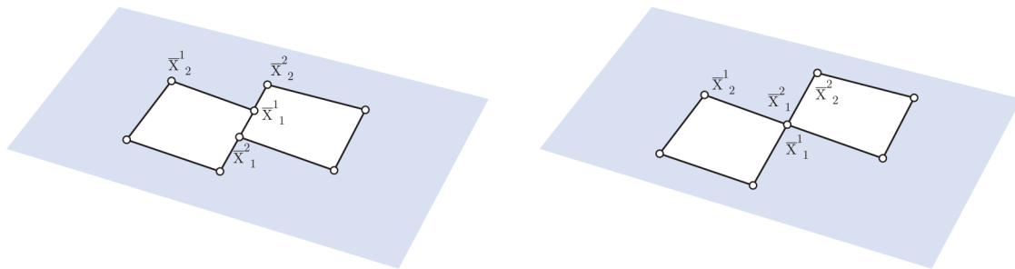
Figure 4.7: Pathological cases within the clipping algorithm
