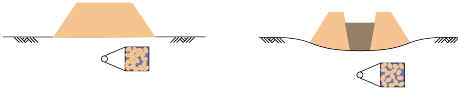
Figure 5.9: Liquefaction phenomena below a dam under a high cycle loading
