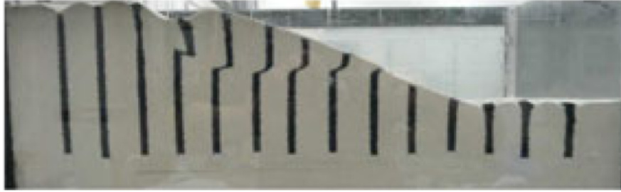
Figure 5.7: Slope stability of a sand specimen under loading on the top (Ehlers and Avci [2012])
