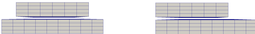
Figure 8.6: Side view of the initial mesh (left) and the end position (right) of the direct shear test with a 3D contact element in between
