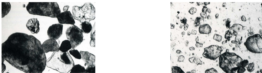
Figure 5.2: Grain characteristic of Karlsruhe (left) and Schlabendorf sand with a higher sphericity (right) given in Herle [1997]
