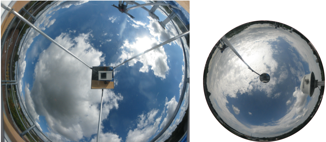
Figure A.2: Sky image from the first spherical mirror system (left). The sky hemisphere was not at the center of the plane mirror and the image did not cover the half space. Image (right) shows the hemispherical result from the second spherical mirror system.
