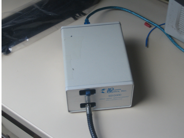
Figure 3.1: The CCD spectroradiometer, SD2000 from Ocean Optics for measuring spectral sky radiance
