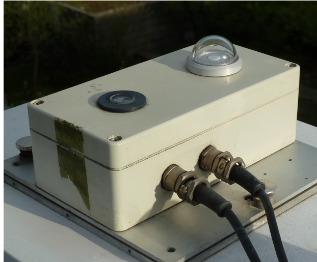
Figure 3.7: The luxmeter measuring the global illuminance manufactured by Czibula & Grundmann on the roof of IMuK [CZIBULA and GRUNDMANN, 2002b].
