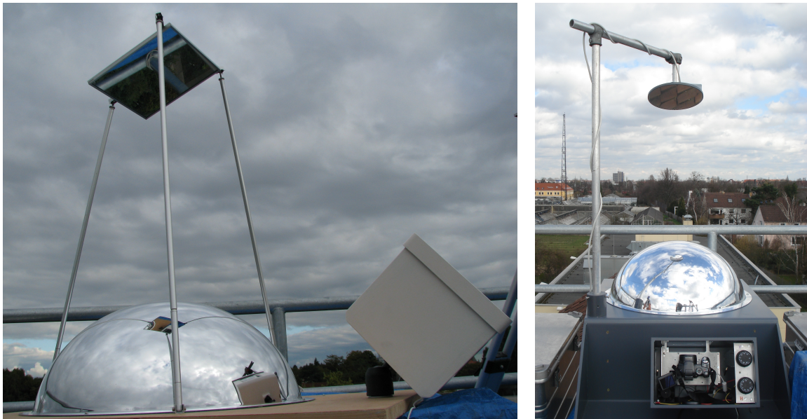
Figure A.1: The final setup of the first spherical mirror system on the roof of IMuK (left) and the white box is the camera housing that contains the camera and its electronics device inside the housing. The second spherical mirror system located on the plastic platform (right).
