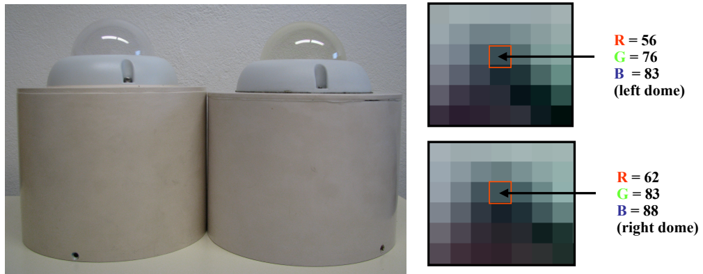
Figure 4.5: Comparison of the new glass dome and the color changing dome. The dome in right hand side appears clearly darker than the other one and when comparing the images taken through the both dome, the color RGB values might be changed, minimum about 5 counts. This can impact on a further colorimetric investigation.
