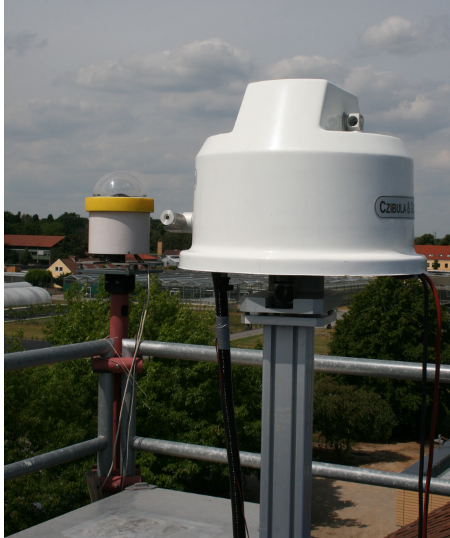
Figure 3.3: The skyscanner on the platform of IMuK. The luminance detector is a small metallic object above the label in the left side. The radiance input optics is fixed to the secondary axis and the optical fibre is attached to the input optics.
