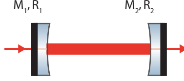
Figure 2.1: Schematic of a Fabry-Perot cavity: The light couples into the cavity through in-coupling mirror M_1 with reflectivity R_1 . The second mirror M_2 with reflectivity R_2 faces M_1 . Between the two mirrors a standing wave develops. The light field is transmitted by the end-mirror M_2 .
