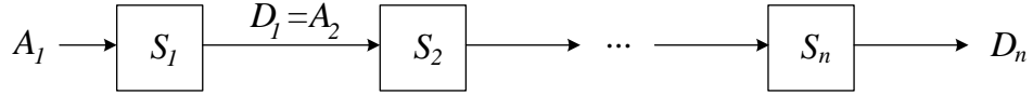
Figure 2.2: A flow traversing a network of tandem nodes with service curves S_i(t) for i \in [1, n] . Traffic arrivals to the network are denoted A_1(t) , while network departures are given by D_n(t) .
