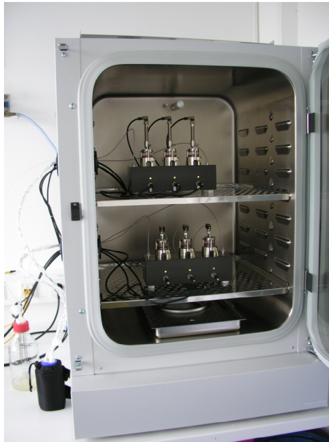
Figure 4-77: Experimental setup for the cultivation of cell cultures grown on insert membranes at the air-liquid interface in the computer-controlled CULTEX® Long Term Cultivation (LTC) system
