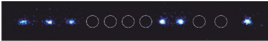
Figure 7.2: Coulomb crystal with {}^{172}\text{Yb}^+ ions fluorescing at 369 nm and sympathetically cooled {}^{115}\text{In}^+ ions (indicated by white circles). The indium ions are confirmed by measuring the mass-dependent secular modes of the crystal via parametric excitation.
