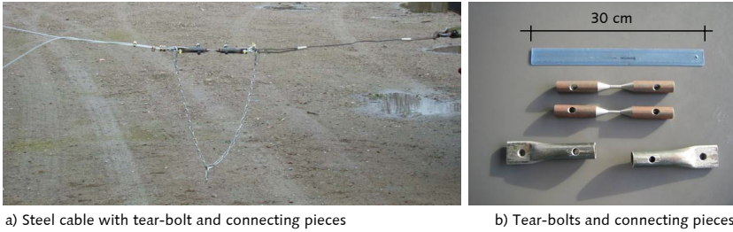
Tear-bolt system with steel cable
