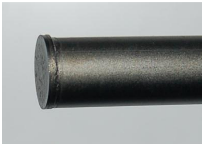
Figure 1.3 Dead-end BSCF tube membrane with an outer diameter of 1 cm and 1 mm wall thickness as produced by the Fraunhofer Institute IKTS Dresden/Hermsdorf (Germany).
