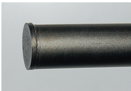
Fig. 1. Dead-end BSCF tube membrane with an outer diameter of 1 cm and 1 mm wall thickness as produced by IKTS.
