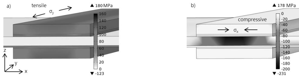
Fig. 5. a) Cross section of the interconnection with the normal stress in y-direction highlighted. b) The same cross section with the normal stress in x-direction.
