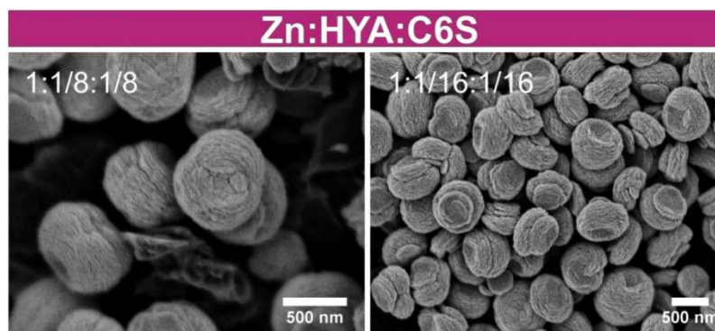
Figure S7: FE-SEM micrographs of zincite superstructures grown for 300 min in a mixed poly-sugar experiment. Both PSs were added in a HYA:C6S:Zn(II) ratio of (1/8):(1/8):1 and (1/16):(1/16):1, respectively.
