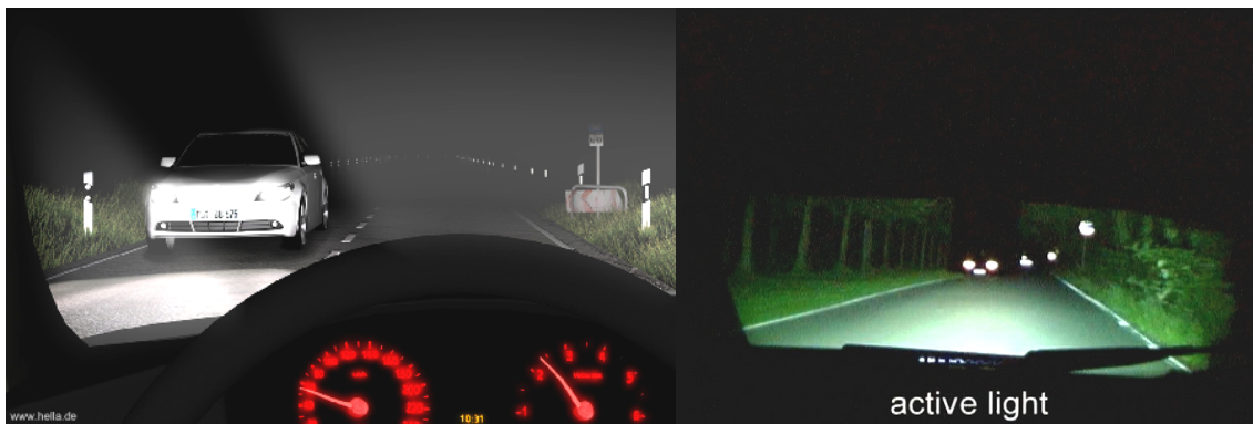
Figure 2.1.3: Left:Concept of The Glare-Free High Beam, Right: Output of The Prototype
