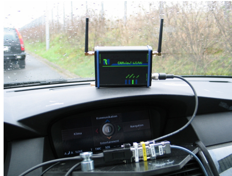
Figure 3.5.5: CAN View WLAN
