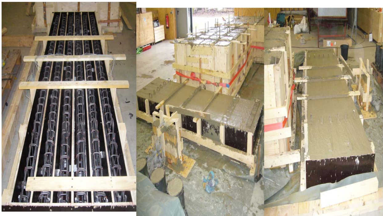
Figure 3-8: Casting of the Part II specimens
