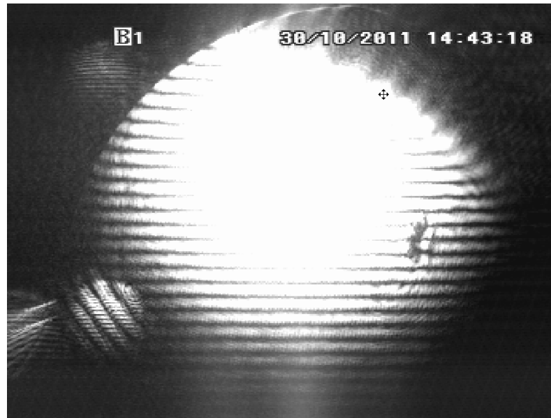
Figure 4.2: Picture of the beam circulating in the interferometer, as seen in transmission of MFE. The horizontal fringes are interference patterns caused by the fact the MCE and MCN are hanging higher than MFE, MFN and the beam splitter.
