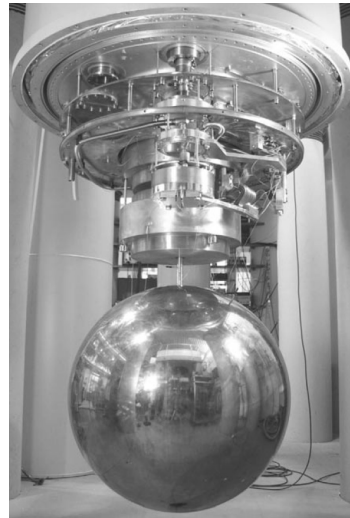
(b) The MiniGRAIL resonant sphere detector at Leiden University (grayscale image) [dWGvH + 03].
