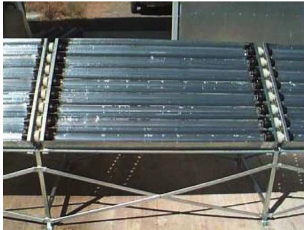
Figure 5: View of one CPC collector module (photo made at PSA, Spain) (Fernández et al., 2005).
