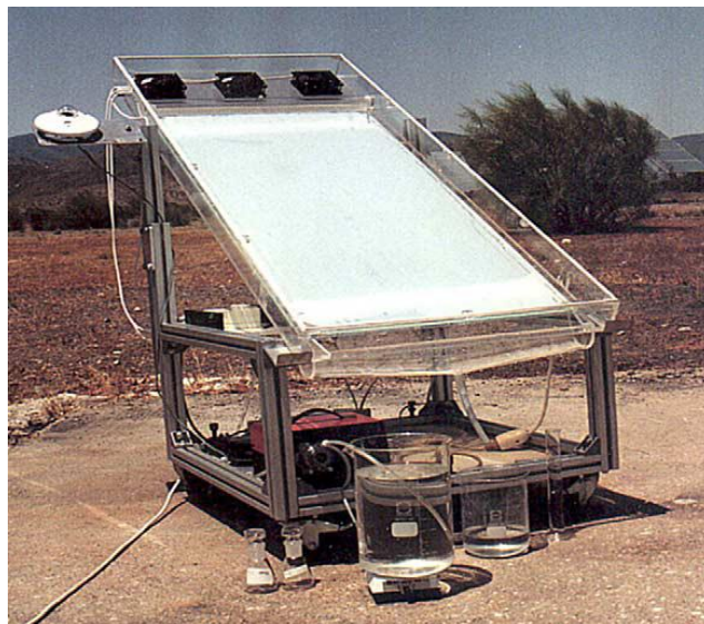
Figure 6: Photograph of the TFFBR reactor installed at the Plataforma Solar de Almeria in Spain (Photo: D. Bockelmann) (Bahnemann, 2004).
