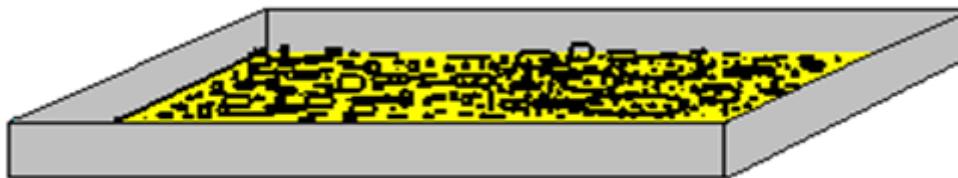
Figure 11: Polypropylene pan filled with 400 g of 5 mm . 5 mm of pellet type photocatalyst
