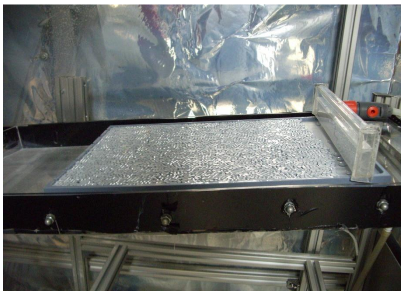
Figure 12: Flat packed reactor, BASF Pellet catalyst size of 5 mm . 5 mm
