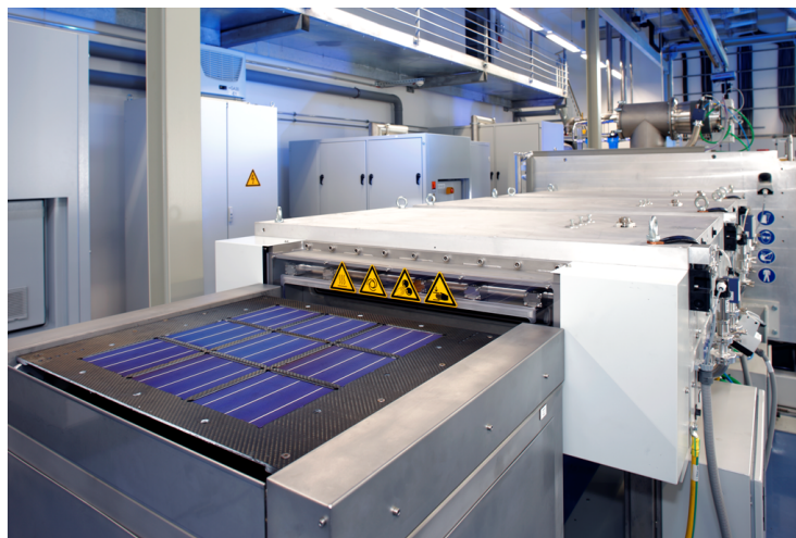
Figure 1.3.: In-line high-rate evaporation system ATON 500. The image shows the unloading area of the system and a carrier with 9 silicon solar cells after the rear side metallization.
