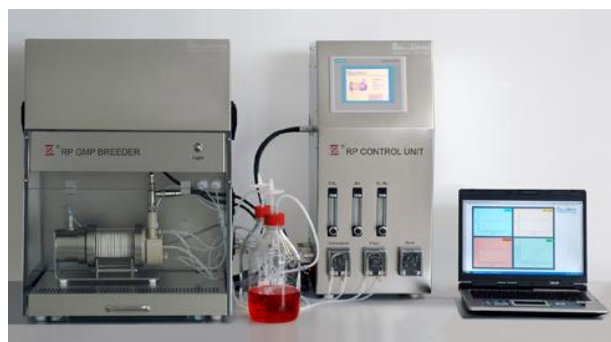
Figure 38: Z@RP 2000 H bioreactor system with breeder and control tower
