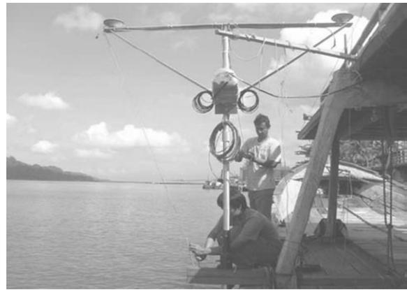
**A7.4 Mounting the F180 at portside-hull**
