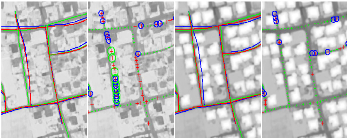
Figure 40. Details of test site 4: two images on the left: without building energy; two images on the right: with building energy (blue line: initialisation; red line: final position; green line: reference centerline; circles: errors detected by the internal evaluation (green: first detector; blue: second detector) ; crosses: image energy lower (green) or higher (red) than the mean value)
