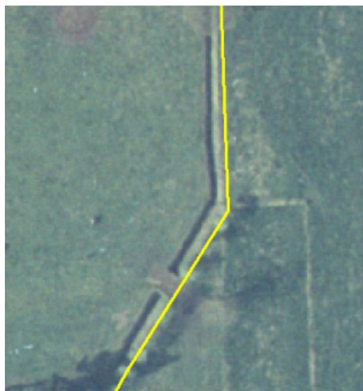
Figure 43. Errors in the GIS river network (test site 2b - detail): background: orthophoto; yellow: ATKIS data
