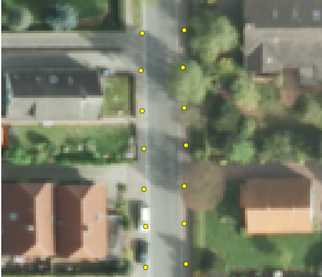
Figure 22: Position of the optimised ribbon borders (yellow points) superimposed to an orthophoto
